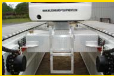
Auxilliary Fuel Tanks with Ladder
